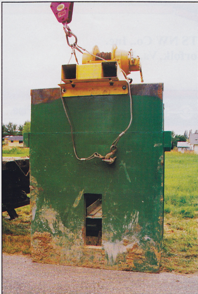
The 200-ton pipe burster used a maximum of 60 tons of pulling force throughout the project.
